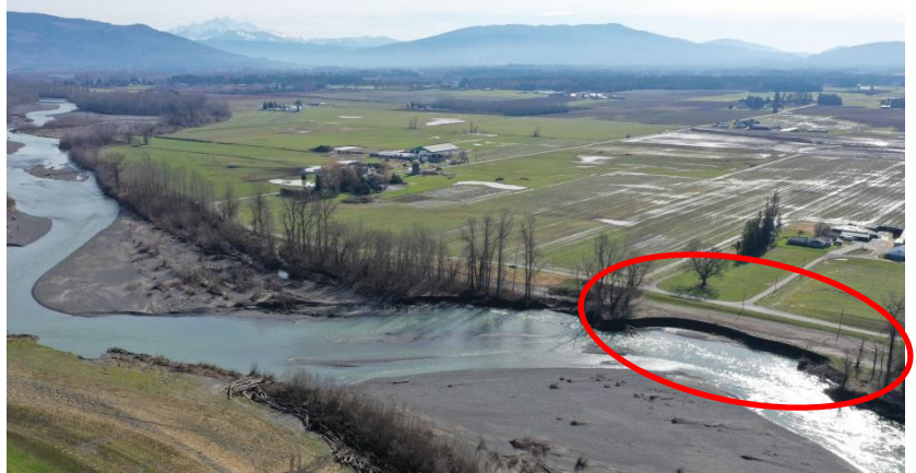
Erosion threatening Abbott Levee and Road
