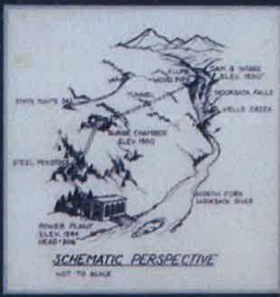
Schematic of the Nooknock Falls Hydroelectric Project
