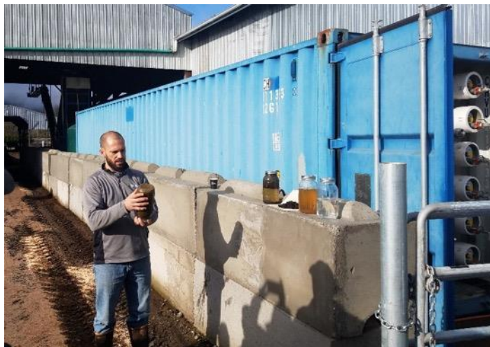
Figure 3.13: Coldstream Dairy Farm has installed a three-stage processing system to manage dairy manure and produce water clean enough to be returned to nearby streams.
