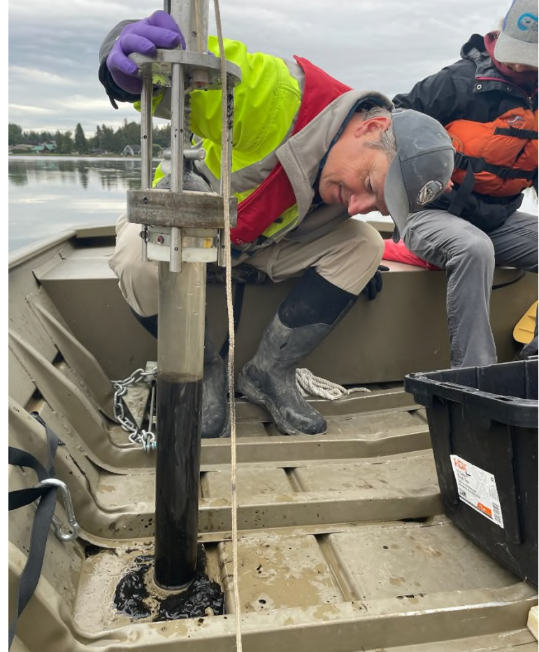
Sediment core sampling on Wiser Lake. Source - WCHCS
