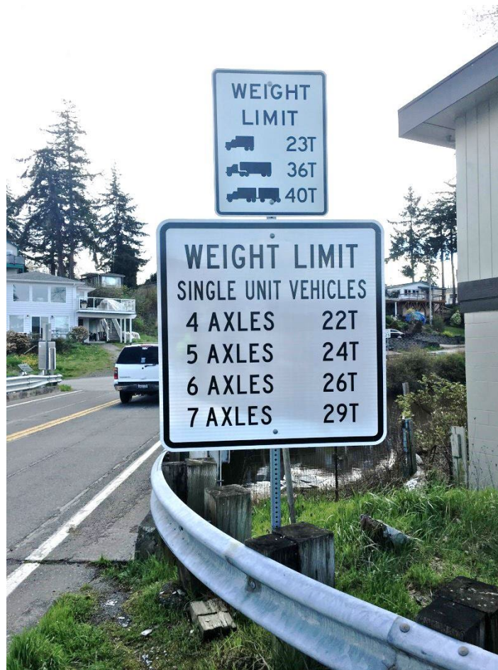
Posted weight restrictions for Jackson Road/Terrell Creek Bridge No. 81 showing AASHTO 1, 2 & 3 and single unit vehicles 4-axles through 7-axles restrictions.
