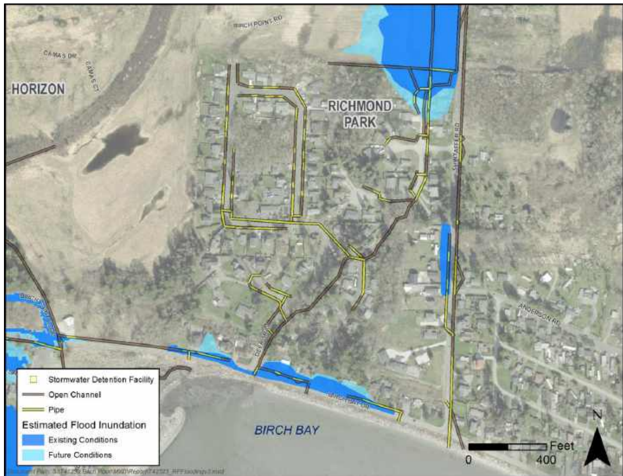
Figure 16. Simulated Flooding in Shintaffer Sub Area - Existing and Future Conditions, November 2021 Event
