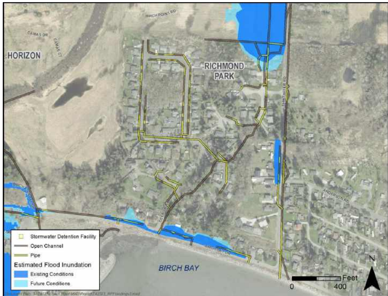
Figure 15. Simulated Flooding in Shintaffer Sub Area - Existing and Future Conditions, 100-year Event
